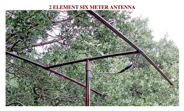
The 6 meter antenna has two elements and is housed in ½ inch pvc tubing, using T connectors to form the yagi configuration, and another T is located mid-way between the two elements for support. End caps are used to enclose the pvc ends. The coax feed is inserted into the DE T via a drilled hole on the T's under From The N3U||.COM Document Library
